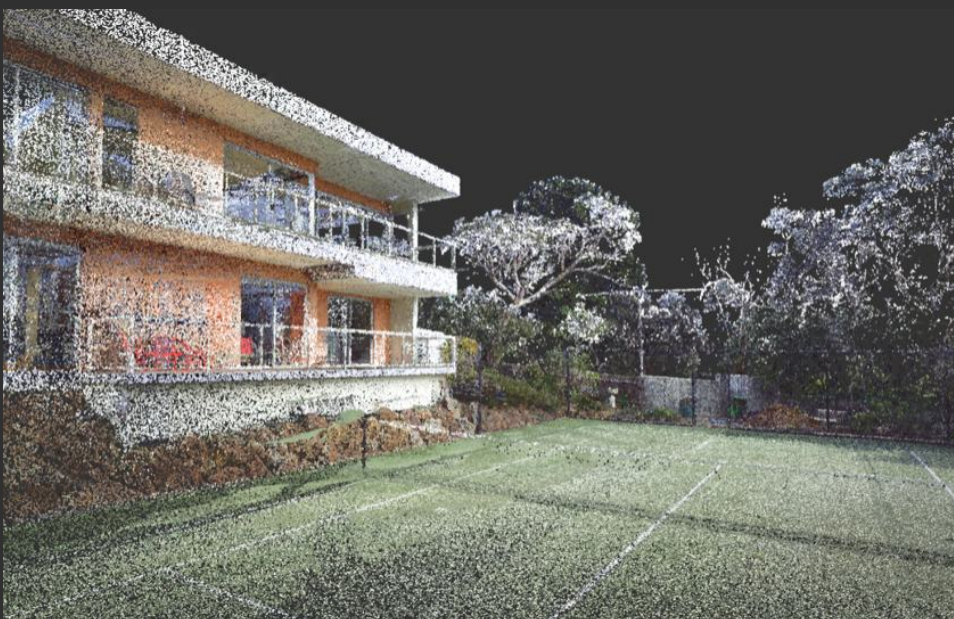
Above image is a 3D laser scanned point cloud that can be imported into architectural software.
